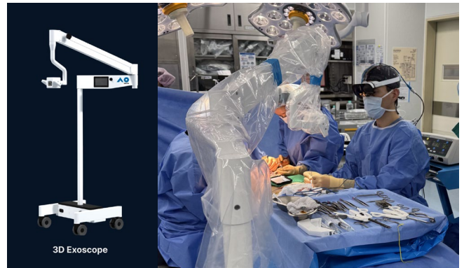
Fig. 1. (Left) HUD-based 3D digital exoscope system (SHIYA, MediThinQ, South Korea) (Right) Intraoperative use of the HUD-based 3D digital exoscope system during microvascular anastomosis.
