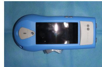
Figure 1. MolecuLight fluorescence imaging device. Representative photograph of the MolecuLight system used for point-of-care fluorescence imaging to visualize bacteria-associated signals in wounds.
